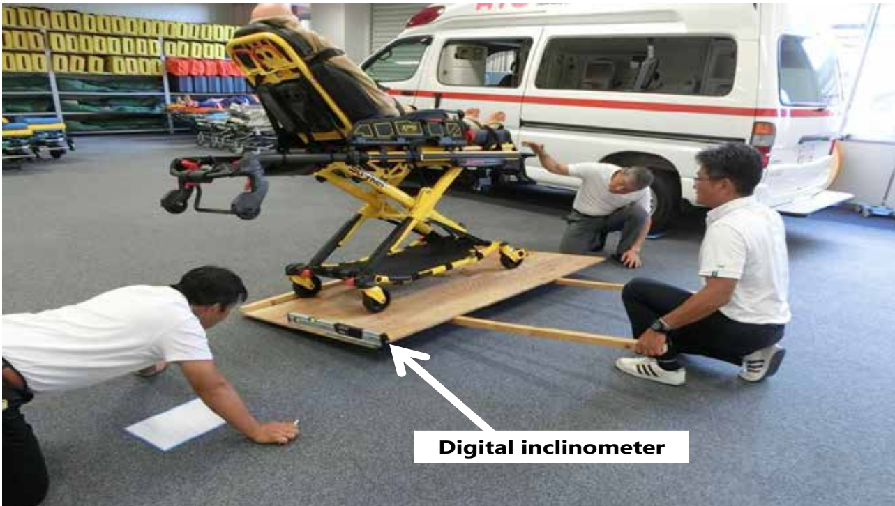
Figure 1: The tipping angles were measured by a digital inclinometer.
