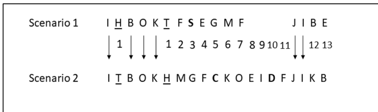
Figure 2. Illustration of Levenshtein distance calculation. In this hypothetical example, the workflow for scenario 1 could be converted to scenario 2 in 13 steps. The underlined activities of scenario 1 (H and T) can be replaced to match scenario 2. Therefore, Scenario 1 can be matched to Scenario 2 by switching H and T. Other edits were changing or adding activities. S was the unique activity in Scenario 1. C and D are the unique activities in Scenario 2.
